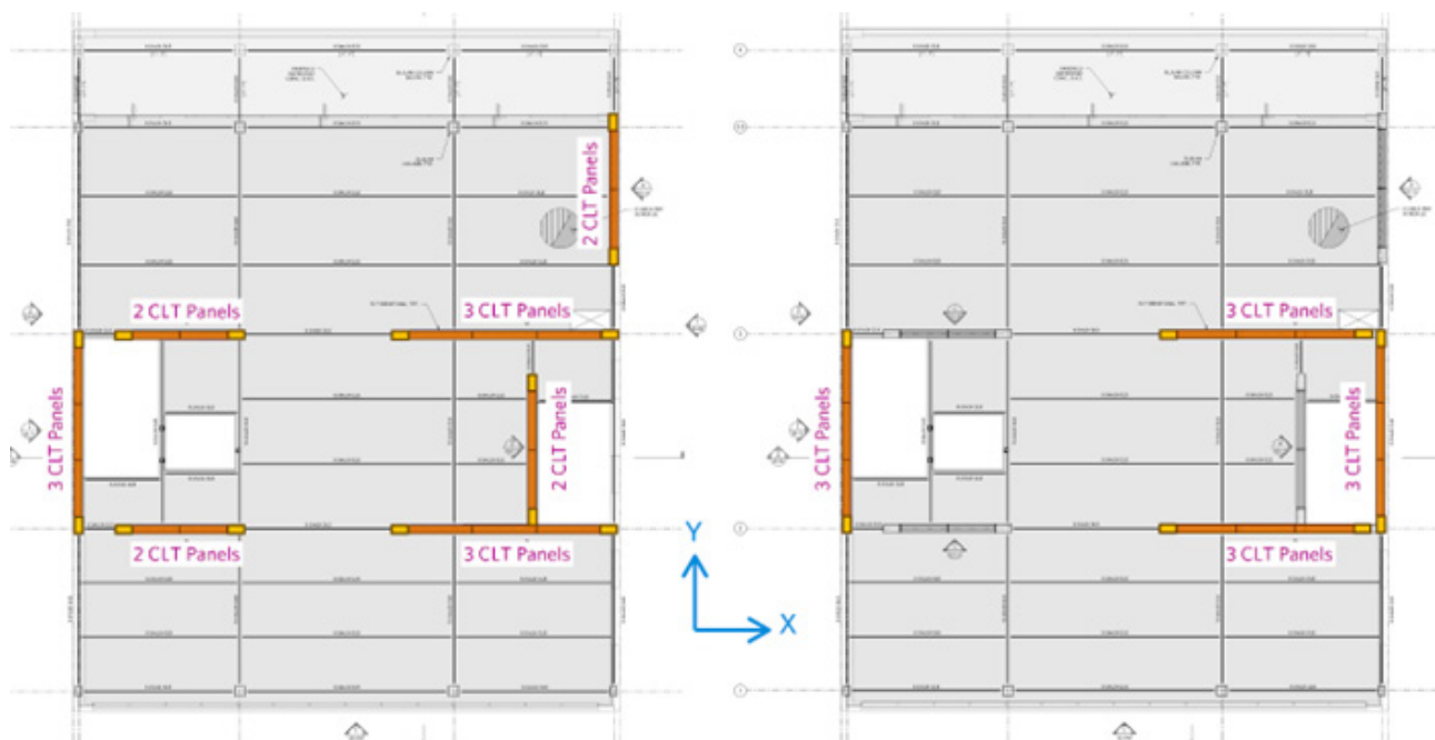
Figure 4 Designed CLT shear wall locations: (a) Limited ductility design (R=4); (b) Optimized design (R=8)
